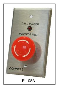
**Description:** E-108A stations feature single-gang stainless steel faceplate with silk-screened designations. The E-108A has a "Mushroom" push-button with mechanical latching. Push on/twist off. They may be flush mounted on standard outlet boxes with single-gang rings, or surface mounted on Wiremold 5748 or equal with a depth requirement of 1 3/4". The activator is oil tight. Momentary switching is available.
