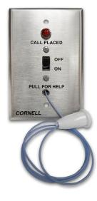
**Description:** E-104-1/E-104-1WP stations feature satin finished stainless steel faceplates with silk-screened designations. Station is applicable for single or dual applications. E-104-1WP has a gasket making the station splash proof for use in shower applications. They may be flush mounted on standard outlet boxes with single-gang rings, or surface mounted on Wiremold 5748 or equal with a depth requirement of 13/4".
