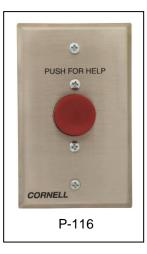
**Description:** The (P-106) (P-116) stations feature satin finished stainless steel faceplates with silk-screened designations. The UL Listed switch is rated at 15 amperes @ 125 volts AC. Momentary action switch can be wired for NORMALLY OPEN or NORMALLY CLOSED function. Three female SLIP-ON connectors are provided.
