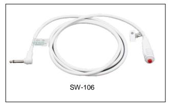
**Description:** A shockproof, plastic housing holds the cord's momentary contact push button operator, connected to a vinyl-covered cord six feet (SW-106) or ten feet (SW-110) long. The right-angle plug is molded to the cord for long life. Bedding clips are included. *Maintenance*: The entire assembly will withstand sterilizing and routine washing.
