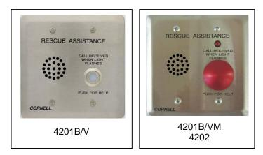
**Description:** The Cornell 4200 series call stations work with Cornell's 4200 Rescue Assistance system to initiate a call to the master panel when the button is pressed, opening up a voice communication from master panel to station.
