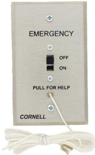
**Description:** The Momentary Emergency Station (E-144) to be used with a latching Annunciator panel features satin finished stainless steel faceplates with silk-screened designations. It may be flush mounted on standard outlet boxes with single-gang rings, or surface mounted on Wiremold 5748 or their equivalents, with a depth requirement of 1 3/4". Field wiring terminations are with pig-tails.
