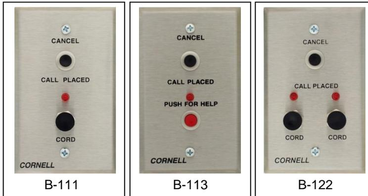
**Description:** UL-listed CORNELL Bedside Stations may be equipped with one or two jacks (B-111, B-122) for use with CORNELL Call Cords, or furnished with push button operations (B-113). Red LED's indicate calls placed. Calls may be cancelled at the touch of a button. Removal of call cord plug from station indicates a call at the system's Annunciator panel.
