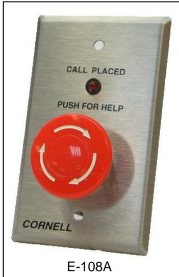
**Description:** E-108A stations feature single-gang stainless steel faceplate with silk-screened designations. The E-108A has a “Mushroom” push-button with mechanical latching. Push on/twist off. They may be flush mounted on standard outlet boxes with single-gang rings, or surface mounted on Wiremold 5748 or equal with a depth requirement of 1 ¾”. The activator is oil tight. Momentary switching is available.
