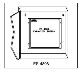
**Description:** The Expansion Switch is designed to accommodate 1-8 devices including Call Stations, other Expansion Switches, or Remote Control Panels. Up to 35 Expansion Switches can be used in the 4800 system to support a total of 255 Call Stations.
