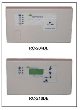
**Description:** The RC-204DE and RC-216DE receiver programs and supervises up to 4(RC-204DE) or 16(RC-216DE) transmitters. Outputs can be configured independently as latching, momentary, or toggle modes. The unit is case tamper resistant, includes jam detection, and houses internal antennas for security. Wireless programming routine is built into the receiver.
