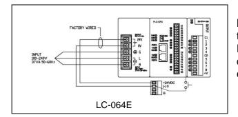
**Description:** The Cornell LC-064E Light Controller to be used with AURA 2.0 has 0-9 flash rate codes. Flash rates are used to determine the priority level of a call, and a different flash rate can be applied to each relay.
