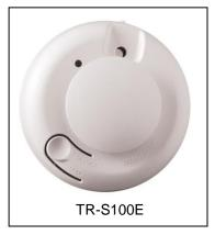
**Description:** The TR-S100E smoke detector utilizes GE Interlogix<sup>™</sup> technology for superior performance, CleanMe<sup>™</sup> diagnostics and improved styling. The TR-S100E is self-monitoring, alerting the user when cleaning is needed, and automatically supervises the radio link to increase reliability. The optical chamber is replaceable, eliminating the need for factory calibration. Suitable for residential applications.
