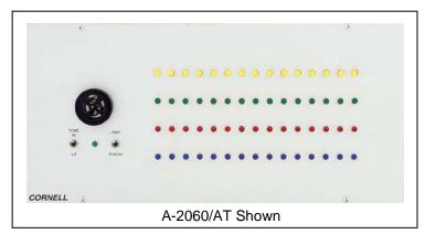
Description: Series 2000 Annunciator panels provide clear indication of all incoming calls. Anodized aluminum finish. Surface or flush mountable. 10, 15 or 25 LED indicators per row are provided for visual alert; an electronic tone, for audible alert. Two tone board operations are available: the (TG) for single status and the (AT) for dual or triple status systems.
