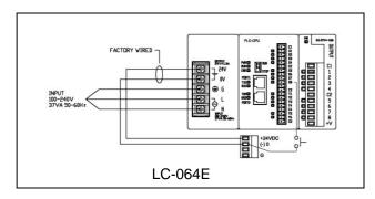
**Description:** The Cornell LC-064E Light Controller to be used with Cornell wireless systems has 0-9 flash rate codes. Flash rates are used to determine the priority level of a call, and a different flash rate can be applied to each relay.
